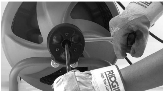
Figure 8 – Autofeed in Reverse Position
