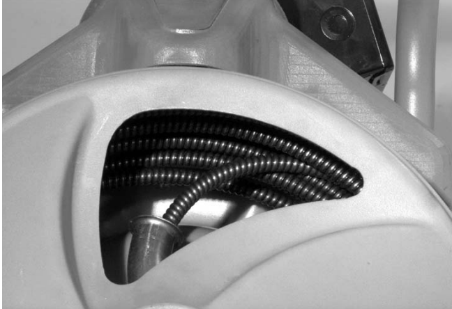
Figure 9 – Coil Cable Into Drum As Shown
