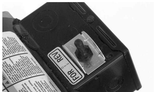
Figure 4 – Directional Switch In OFF Position
