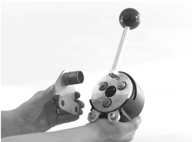
Figure 2 – Placing Mounting Bracket Into Auto Feed
