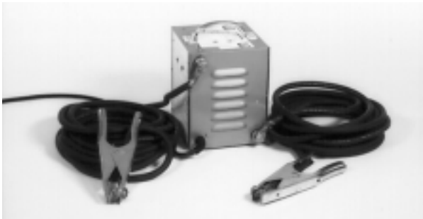
Figure 3 – Thawing Tool with Cables Installed
