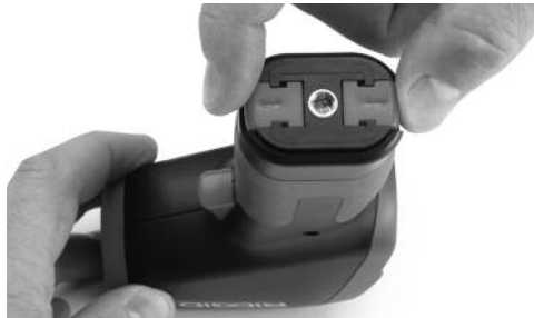
Figure 4 – Removing Battery Compartment
