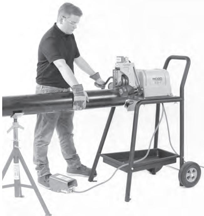
**Figure 16 – Applying Pressure on Pipe**
