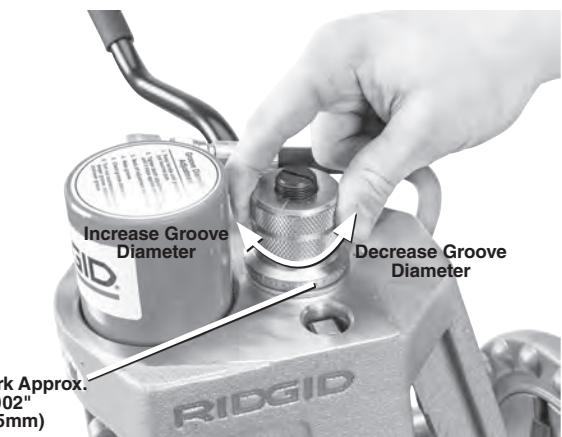
Figure 13 – Depth Adjustment Nut Setting
