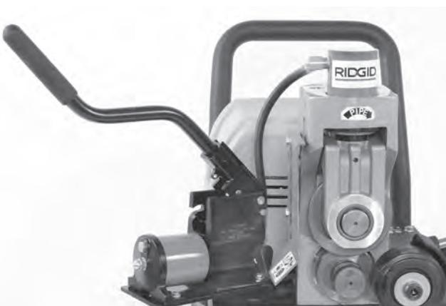
**Figure 7B – Pump in Transport Position [Up]**
