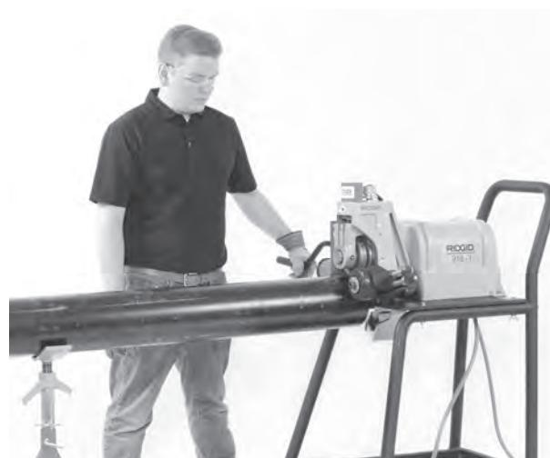
Figure 15 – Proper Operating Position
