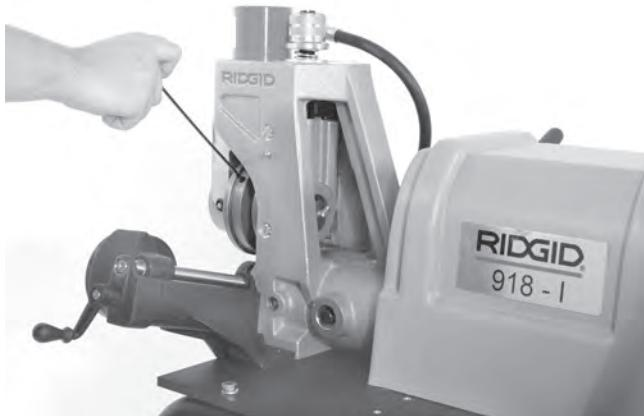
Figure 20 – Loosening Grooving Roll Set Screw
