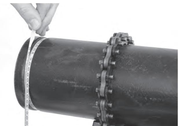
**Figure 17 – Checking Groove Diameter with a Diameter Tape**
