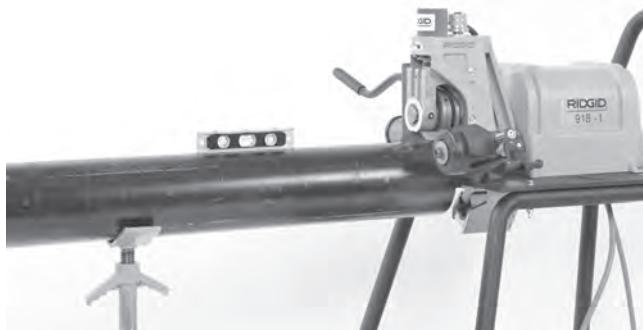
Figure 11 – Leveling Pipe
