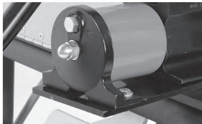
Figure 19 – Reservoir Filler Cap
