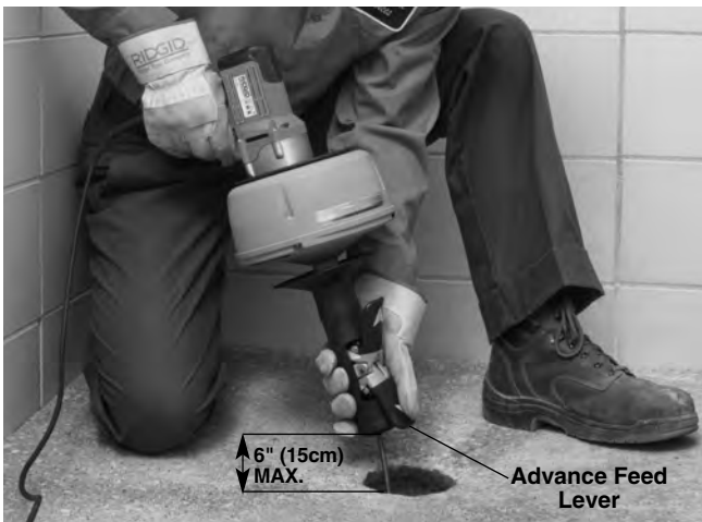
Figure 10 – Feeding Cable With AUTOFEED
