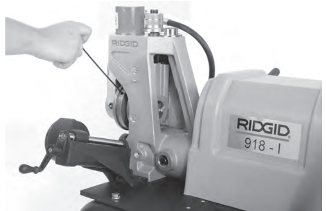
Figure 21 – Loosening Grooving Roll Set Screw
