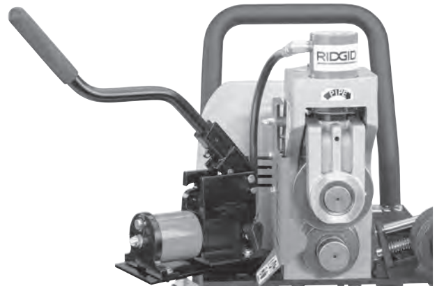
Figure 7B – Pump in Transport Position [Up]
