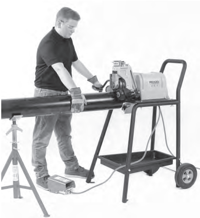
Figure 17 – Applying Pressure on Pipe
