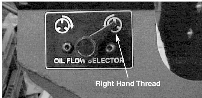
**Figure 24 – LH or RH Oil Flow Selector**
