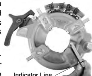
**Figure 14 – Inserting Dies**
