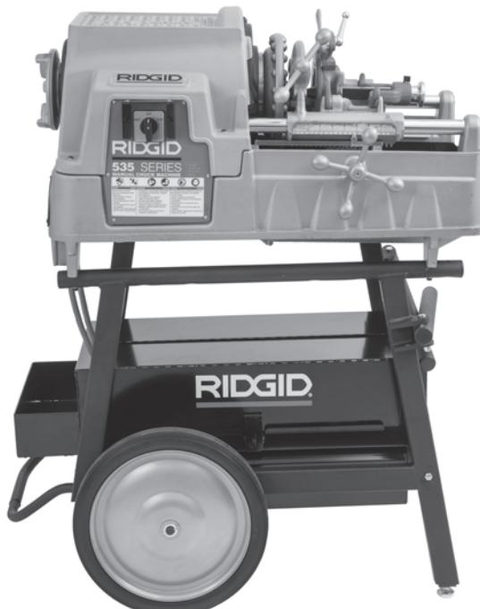
Figure 28 – Machine prepared for Transport
