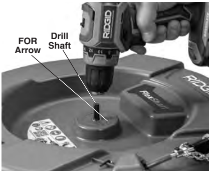
Figure 4 – Attaching Drill To Drill Shaft
