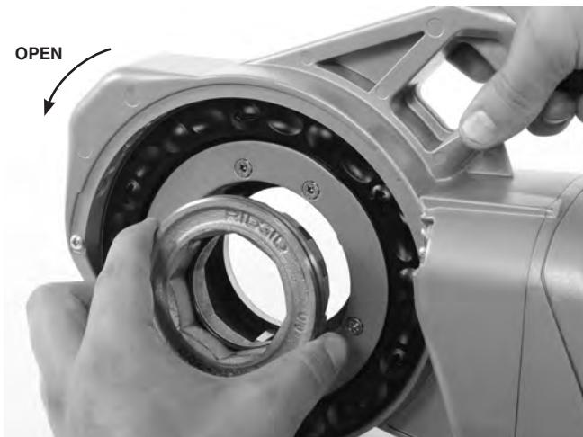
Figure 7 – Installing Adapter
