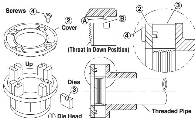
Figure 17 – Installing Dies In Die Head
