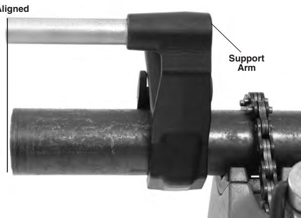
**Figure 10B – Positioning the Support Arm**
