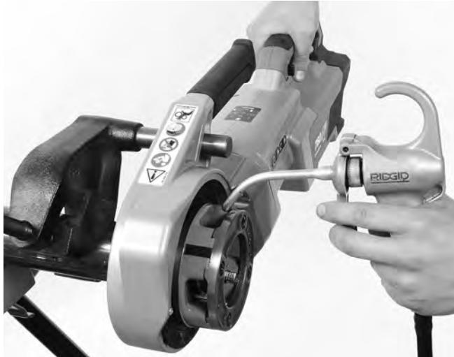
**Figure 14 – Threading Pipe**
