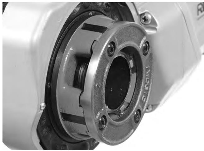
**Figure 15 – Pipe Even with Edge of Dies**
