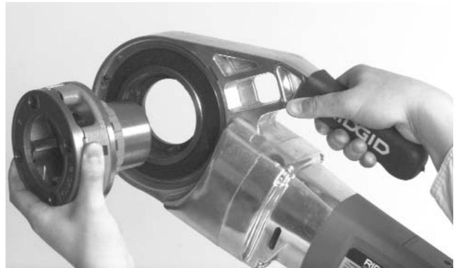
Figure 3 – Installing No. 11-R Die Heads
