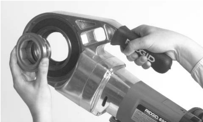
Figure 2 – Installation of 11-R Die Head Adapter
