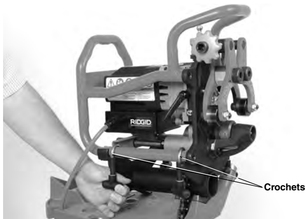
Figure 9 – Securing Beveler to Adapter
