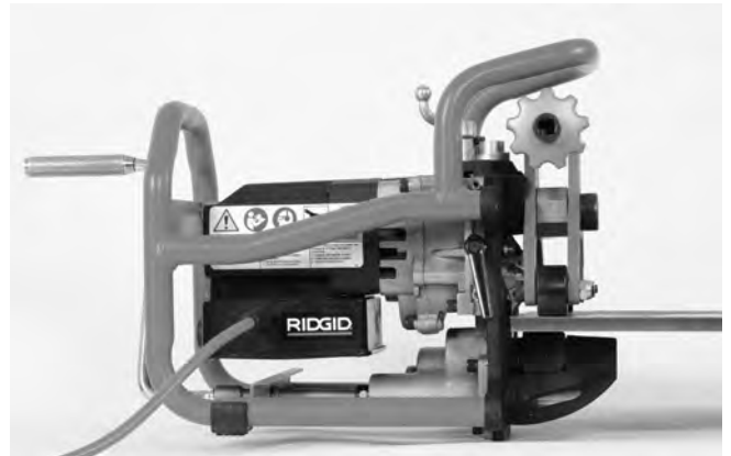
Figure 16B – Installing Beveller on Plate
