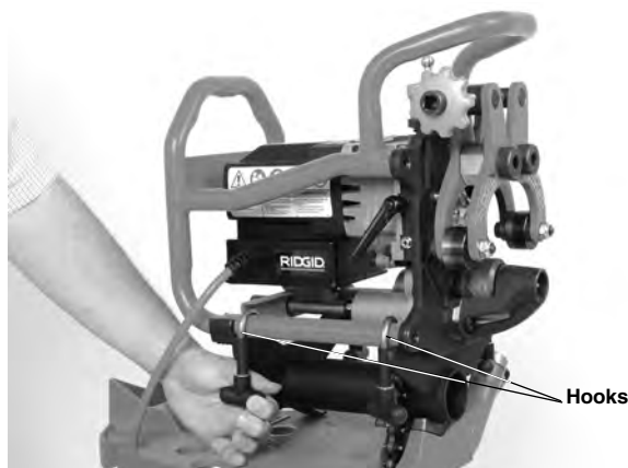
Figure 9 – Securing Beveller to Adapter
