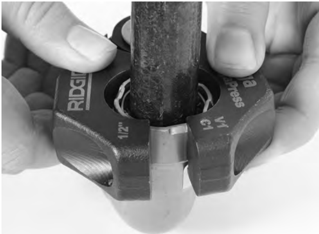
Figure 11 – Installing Press Ring Onto Fitting
