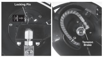
Figure 15 – Reel Brake Adjustment
