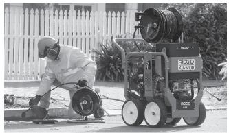
Figure 12 – Proper Operating Position
