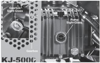
Figure 16 – Checking Pump and Gearbox Oil Level
