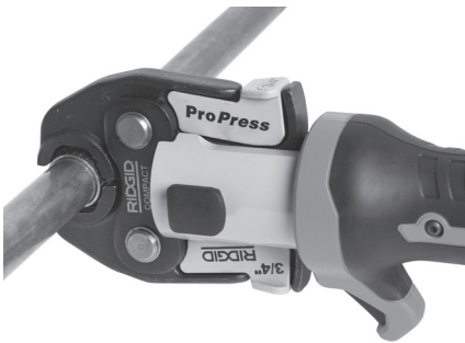
Figure 7 – Placing Scissor-Style Jaws Around Fitting
