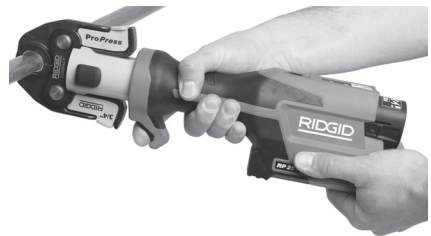
Figure 9 – Pressing the Fitting
