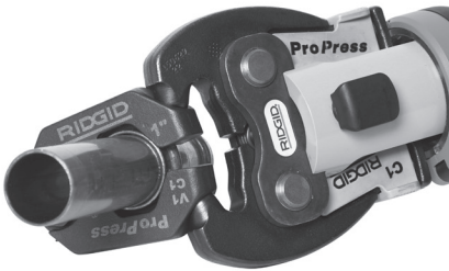
Figure 10 – Attaching Actuator to Press Ring
