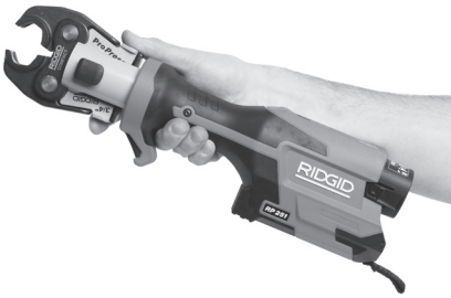
Figure 6 – Opening Jaw with One Hand
