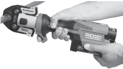
Figure 9 – Sertissage du raccord
