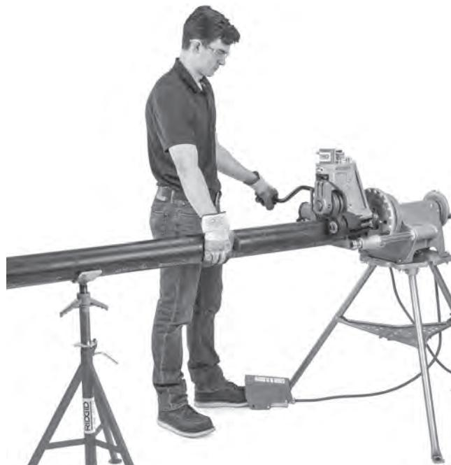
**Figure 20 – Applying Pressure on Pipe with Power Drive in REV direction**
