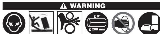
**Keep hands away from grooving rolls. Do not wear loose fitting gloves. Fingers can be crushed between groove rolls, groove roll and pipe or between pipe and stabilizer wheel.**
