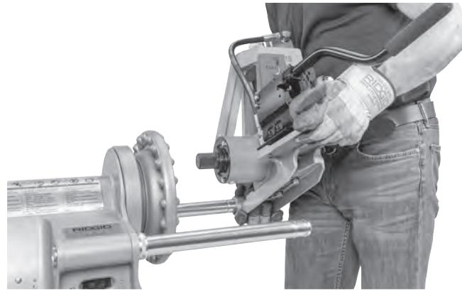
Figure 7A – Installing 918 on 300 Power Drive
