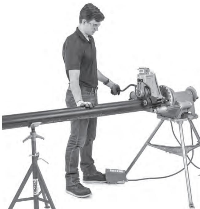
**Figure 21 – Applying Pressure on Pipe with Power Drive in FOR direction**
