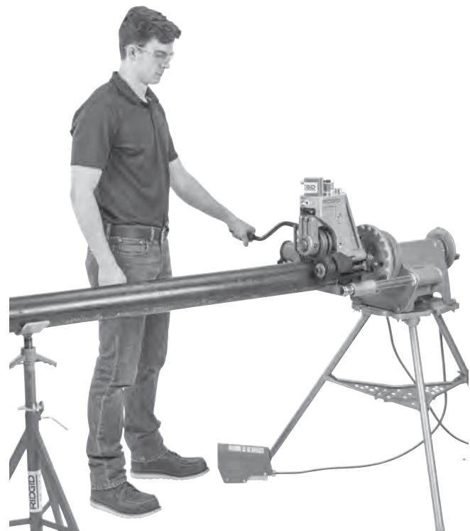
Figure 19 – Proper Operating Position
