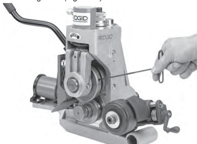
**Figure 25 – Loosening Grooving Roll Set Screw**
