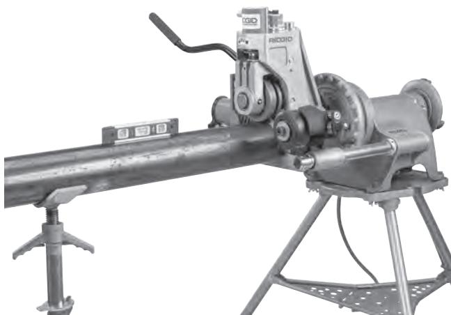
Figure 14 – Leveling Pipe
