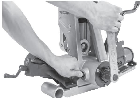
**Figure 29 – Engaging Spindle Lock and Loosen Draw Bolt**
