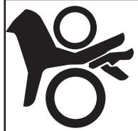
**Do not use this roll groover with a power drive/threading machine that does not have a foot switch.**
