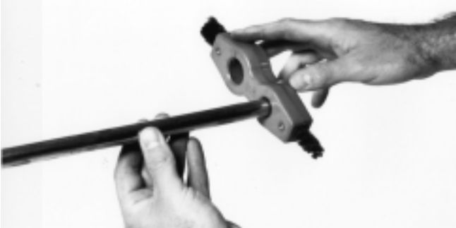
Figure 3 – Cleaning Copper Tube and Fittings
