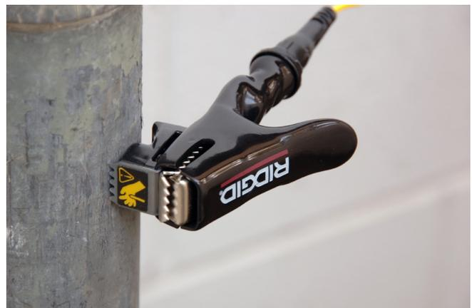
Figure 7 – Connecting the ST-305 using the magnet
