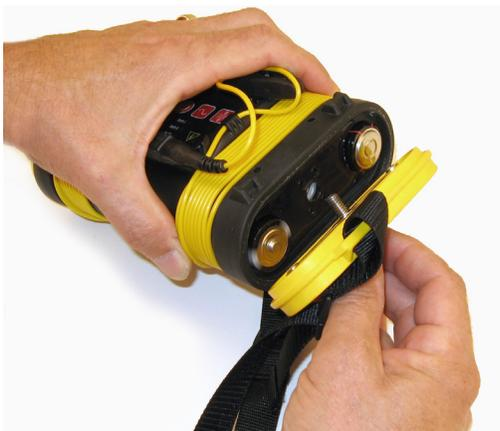
**Figure 4 – Removing the Battery Cover**
