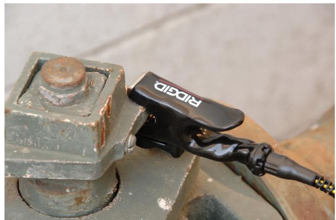
Figure 6 – Connecting the ST-305 using the clip
