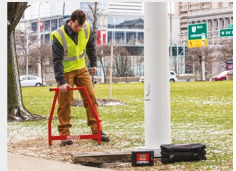
Standard Equipment: FR-30 A-Frame Receiver, FT-103 Transmitter, ground stake, red and black test leads, carry cases, batteries, operator's manual pack
