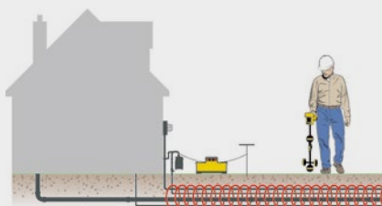
Direct connect to utility lines.
