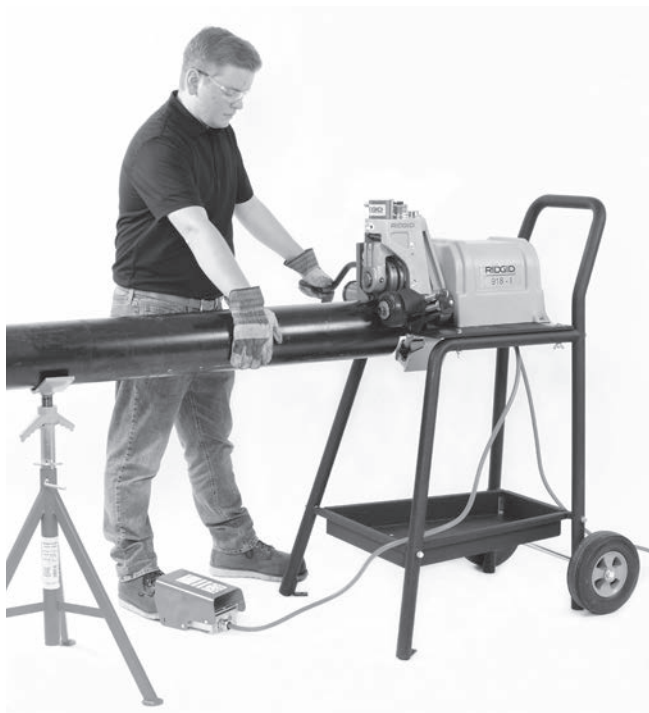
Figure 17 – Applying Pressure on Pipe
