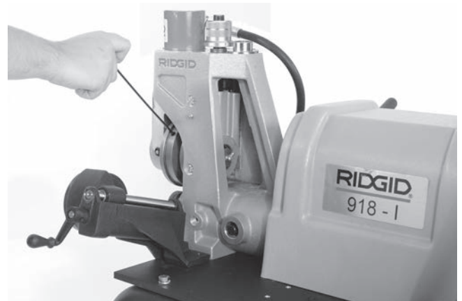
Figure 21 – Loosening Grooving Roll Set Screw
