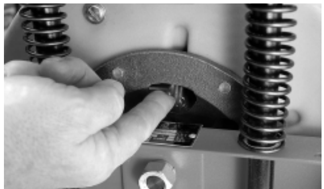
Figure 4 – Lift release pin UPWARD to release drum lock mechanism
