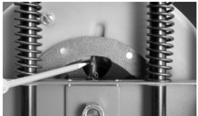
Figure 3 – Rotate drum so release pin is easily accessible
