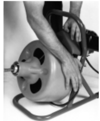
Figure 2 – With belt tension released, slip belt off drum
