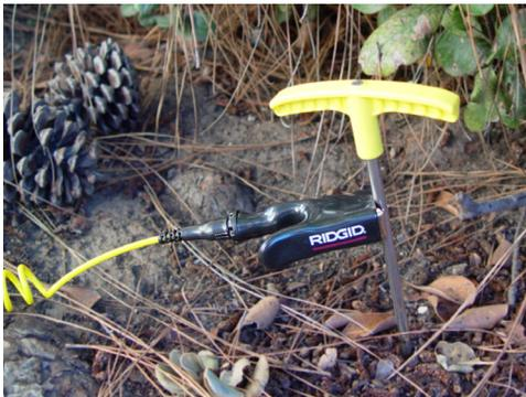
Instead of using the provided grounding stake, the lead clip can be attached to other objects such as a shovel blade or a metal rod sunk into the earth. Using larger grounding objects may improve grounding by increasing the surface area in contact with the earth.
