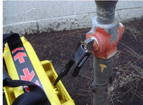
Good contact between the cable lead and the target conductor lowers the resistance of the circuit and produces a stronger tracing signal.
