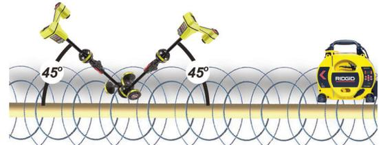
Alternatively, test for air-coupling by standing 6 m [20 ft] away from the ST-33Q+. With the lower antenna on the ground, take note of the indicated depth measurement on the receiver. Raise the receiver vertically 45 cm [18 in] and observe the change in the depth indication. If the receiver only reads the conductor, the depth should increase accordingly. If the receiver is air-coupling, the depth indication will not change by 45 cm [18 in], but will change disproportionately.
