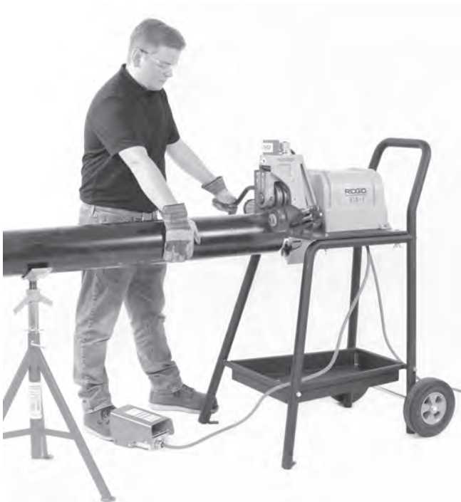
Figure 16 – Applying Pressure on Pipe
