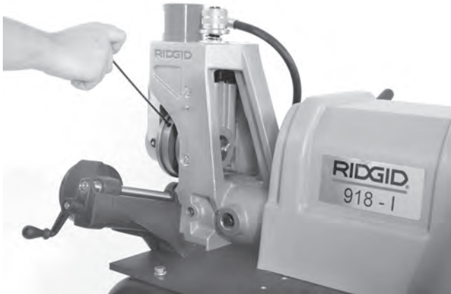
Figure 20 – Loosening Grooving Roll Set Screw
