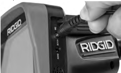
Figure 6 – Powering the Unit with AC Adapter
