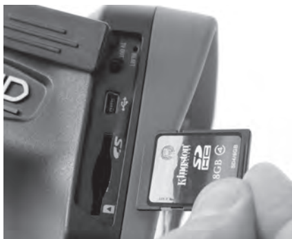
Figure 9 – Inserting the SD Card
