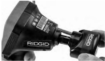
Figure 18 – Camera Connector Plug Installed
