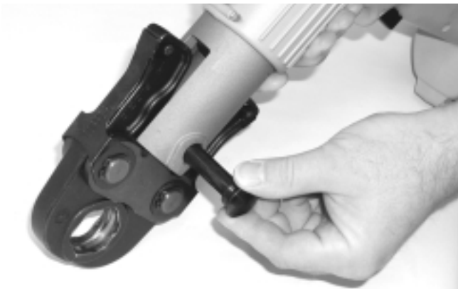
Figure 2 – Pulling The Jaw Set Mounting Pin Out
