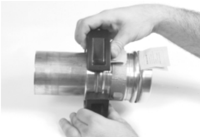
Figure 10 – Installing Press Ring Onto Fitting
