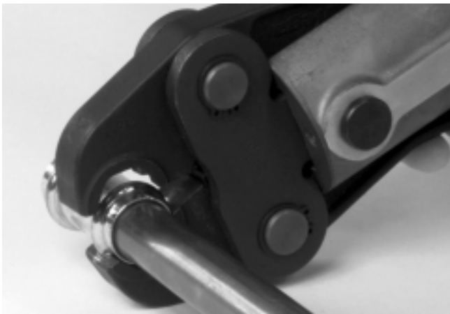
Figure 8 – Placing Scissor-Style Jaw Set Around Fitting
