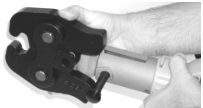
Figure 6 – Sliding RIDGID R2 Ring Actuator Into 320-E
