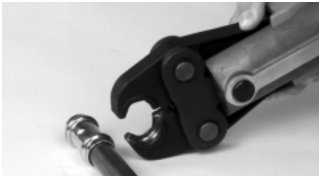
Figure 7 – Opening The Scissor-Style Jaw Set
