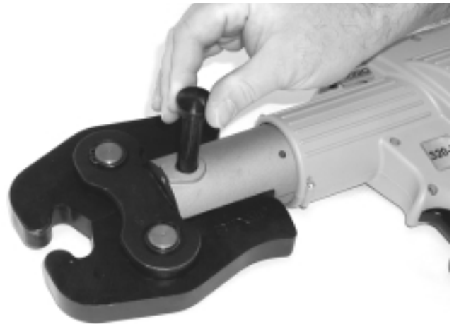
Figure 5 – Pulling The Jaw Set Mounting Pin Out
