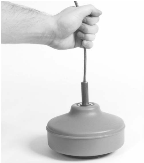
Figure 17 – Feeding Cable Into Drum
