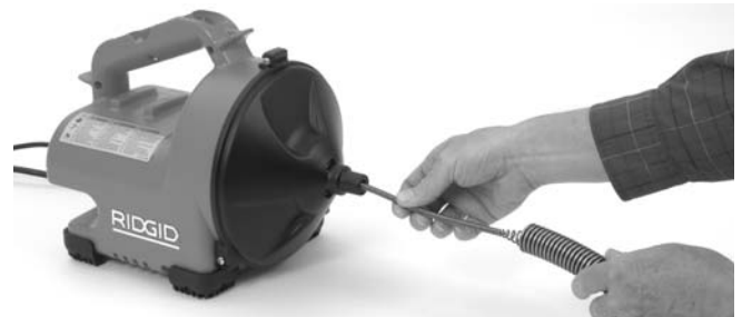
Figure 3 – Feeding Cable into Guide Hose
