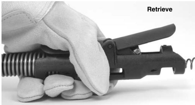
Figure 14B – AUTOFEED in Retrieve Position
