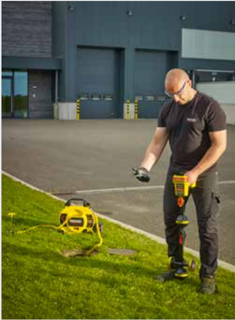
Use the SR-24 receiver to wirelessly change the transmitted frequency on the ST-33Q+ transmitter.
