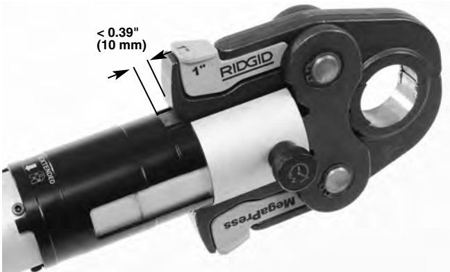
Figure 6B – Fully Closed Attachment Mounting Pin
