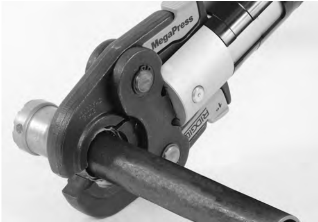
Figure 8 – Placing Jaws Around Fitting
