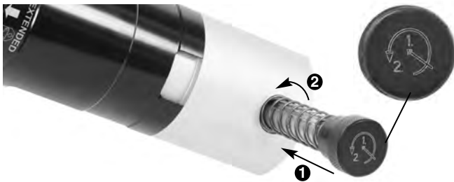
Figure 6A – Fully Open Attachment Mounting Pin
