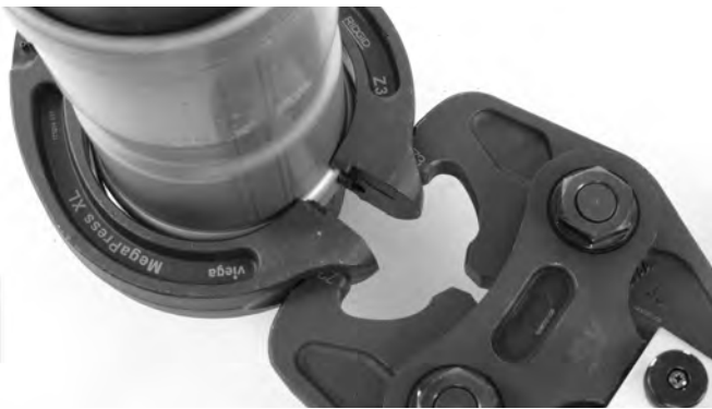
Figure 11 – Attaching Actuator to Press Ring
