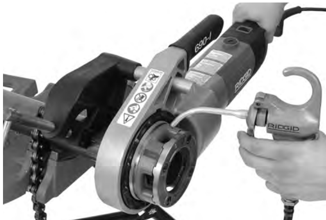
Figure 14 – Filetage du tuyau
