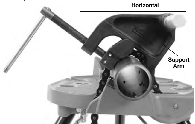
Figure 11A – Positioning the Support Arm
