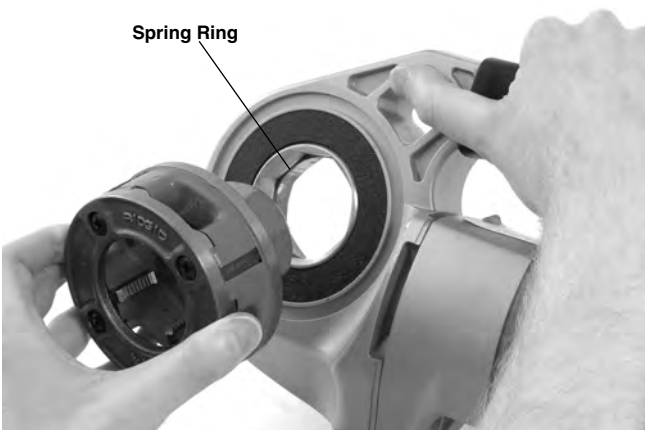
Figure 9 – Installing Die Heads into 600-I Power Drive
