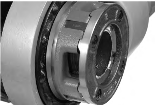
Figure 15 – Pipe Even with Edge of Dies
