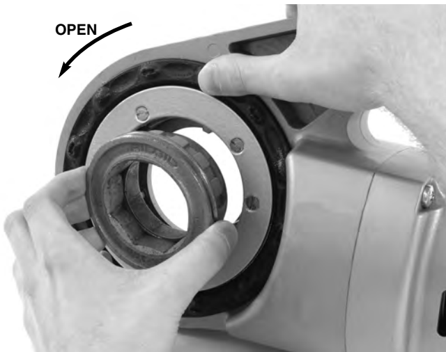
Figure 8 – Installing Adapter Into 690-I
