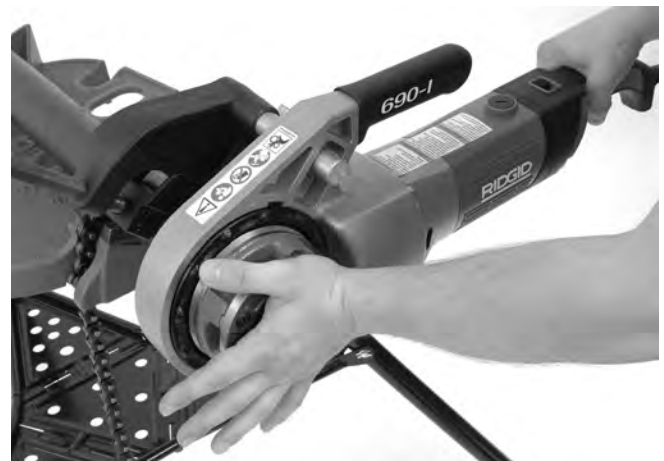
Figure 13 – Starting the Thread
