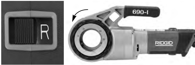
Figure 6B – R (REVERSE) (Counter-Clockwise) Switch Position
