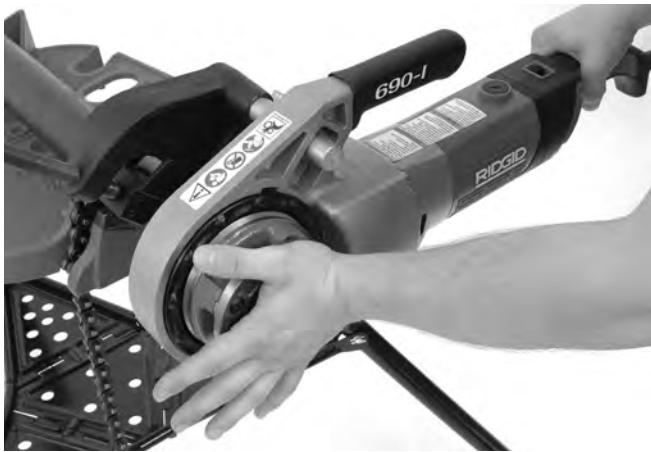
Figure 13 – Entamer le filetage
