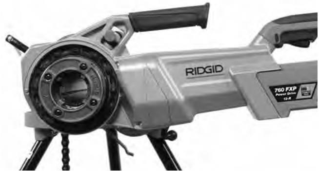
Figure 11 – Orientation appropriée du 760 FXP Power Drive
