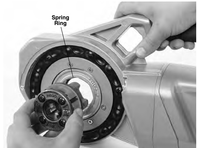
Figure 8 – Installing 1¼" or Smaller 11-R Die Heads (760 FXP 11-R only)
