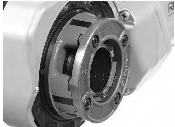
Figure 15 – Pipe Even with Edge of Dies
