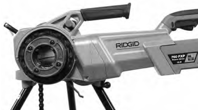
Figure 11 – Proper Orientation of the 760 FXP Power Drive
