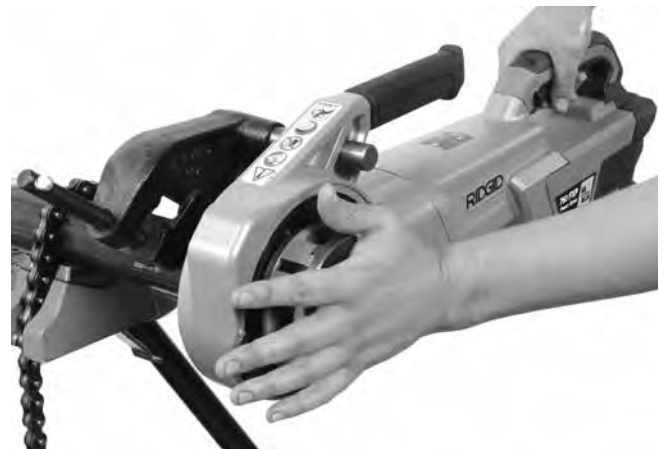
Figure 13A – Starting the Thread Using the Die Head Cover Plate
