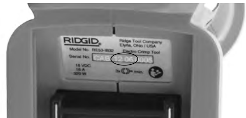
Figure 4 – Machine Serial Number - The first 4 digits (circled) indicate the year and month of manufacture. (12 = year, 06 = month).
