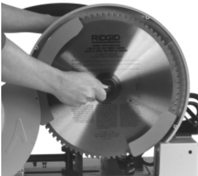
Figure 9 – Installing Saw Blade
