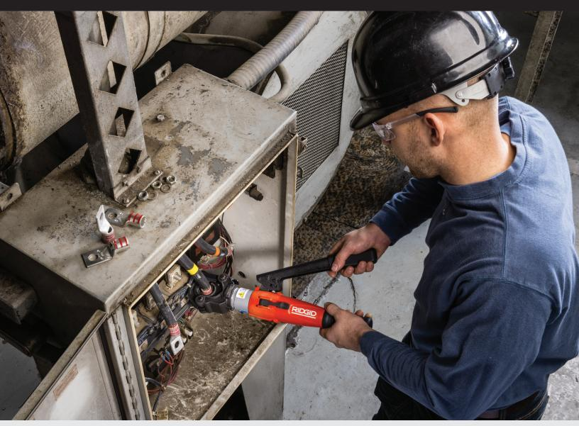
Low handle force and RapidAdvance<sup>™</sup> technology maximize productivity when crimping up to 600 kcmil (MCM) Copper and 350 kcmil (MCM) Aluminum.
