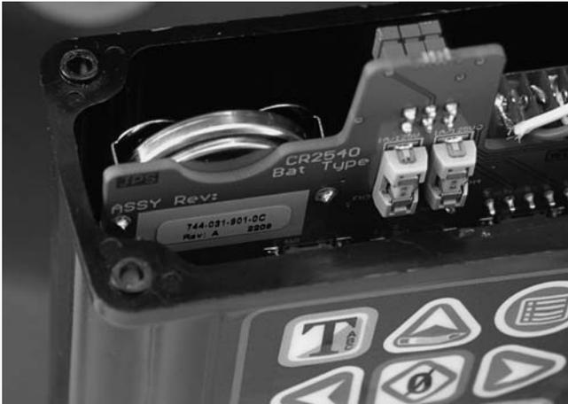
Figura 40 – Pila del CountPlus
