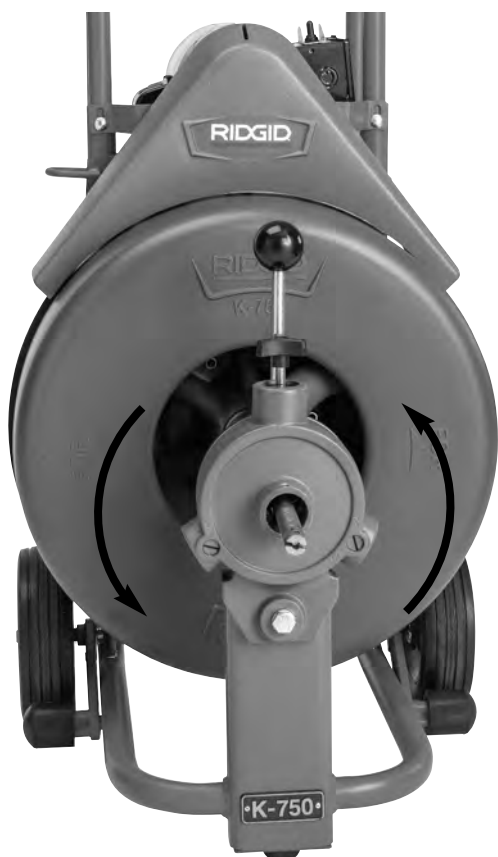
Figure 8 – Proper Drum Rotation (FOR Switch Position)
