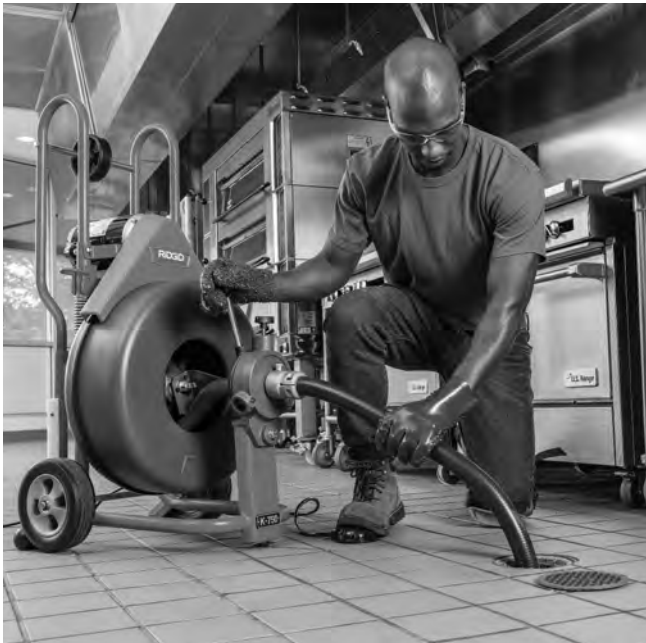
Figure 15 – Using Machine with Guide Hose
