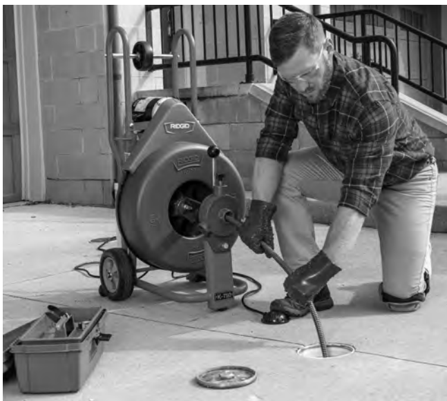
Figure 12 – In Operating Position, Manually Feeding Cable
