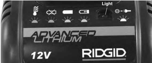
Figure 5 – Charger LED Light and Markings
