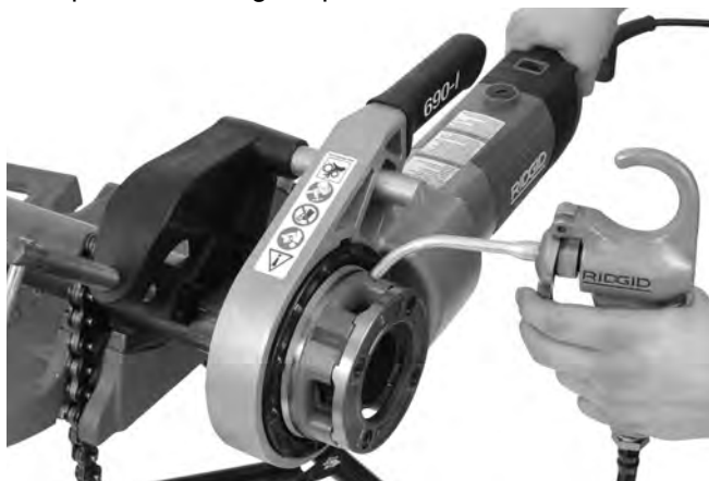
Figure 14 – Filetage du tuyau
