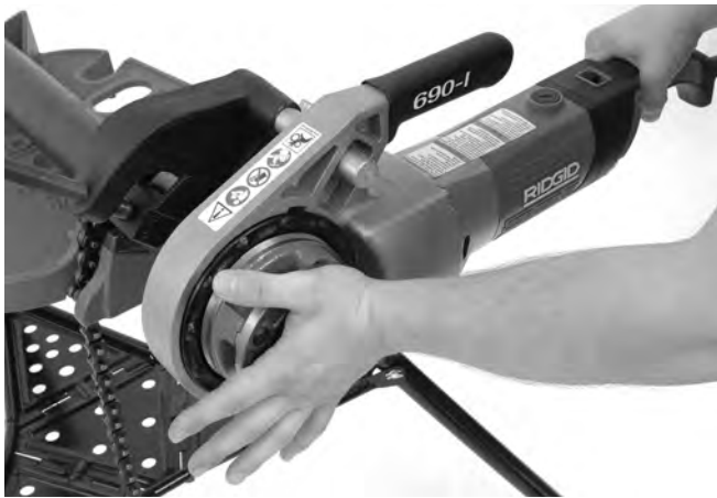
Figure 13 – Entamer le filetage
