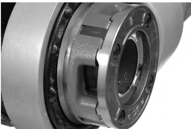
Figure 15 – Pipe Even with Edge of Dies
