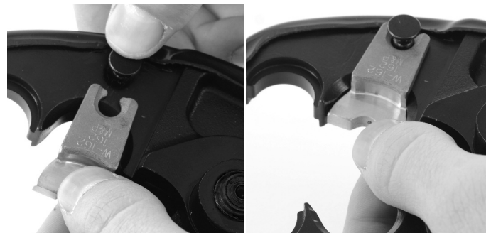
Figure 2 – Installing Dies in Crimp head
