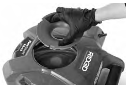
Figur 7A – Ta bort locket
