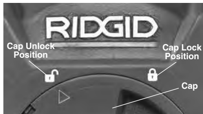
Figure 6 – Unlock the Cap
