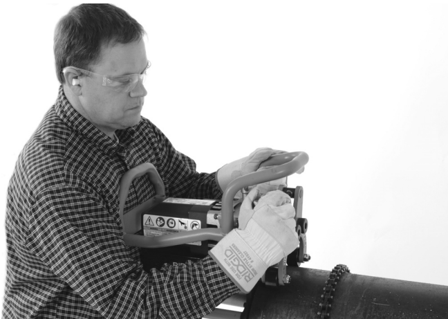
Figure 17A – Hand Tighten Clamp Screw
