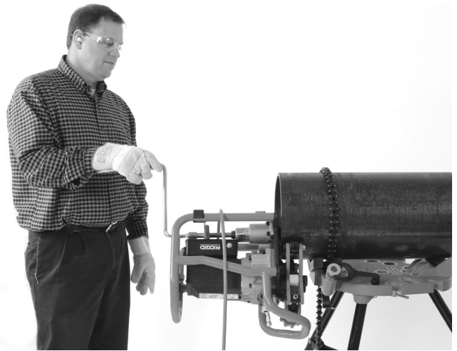
Figure 20B – Bevelling Operation (Fixed Workpiece/Moving Beveller)
