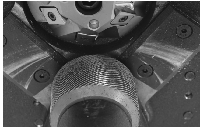
Figure 22– Clean Drive Roll Knurls
