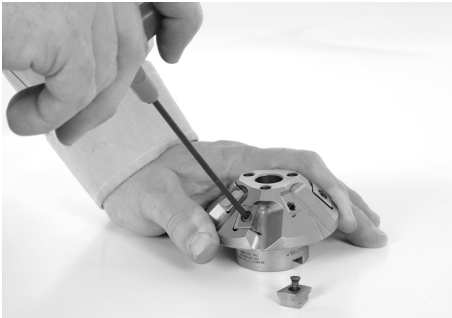
Figure 24 – Replacing Cutter Inserts
