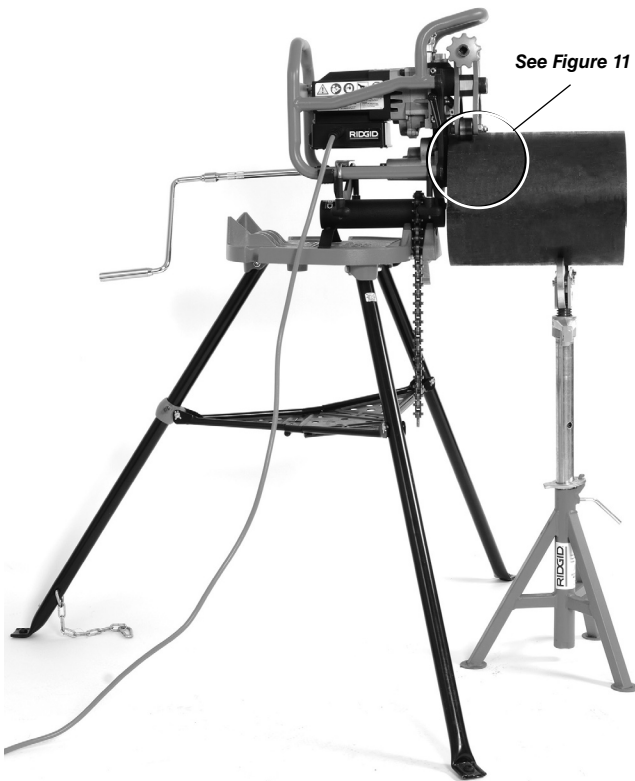
Figure 12 – Fixed Beveller, Short Pipe, One Pipe Stand
