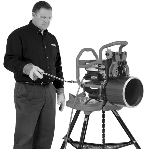
Figure 20C – Bevelling Operation (Fixed Beveller/Rotating Pipe)
