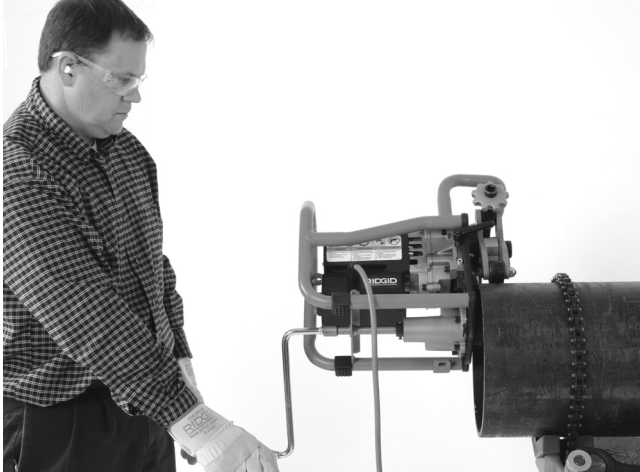
Figure 20A – Bevelling Operation (Fixed Workpiece/Moving Beveller)
