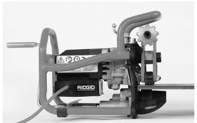
Figure 16B – Installing Beveller on Plate
