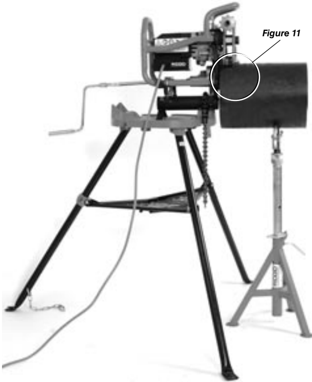
Figure 12 – Machine fixe, tuyau court, un porte-tubes
