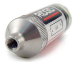
Figure 2 – to install the transmitter onto a push cable, screw the threaded end of the battery cover onto the end of the push cable. Tighten with pliers to make sure it doesn't work loose during use.
