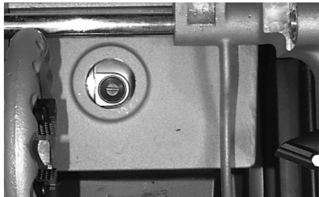
Figure 19 – Brush Cap Plug Removed, Brush Holder Exposed
