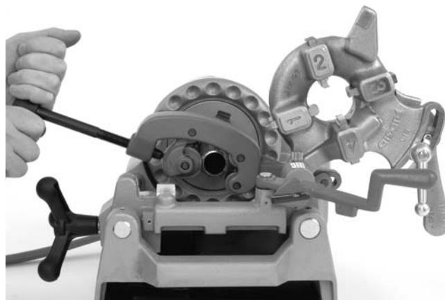
**Figure 11 – Cutting Pipe with No. 354 Cutter**
