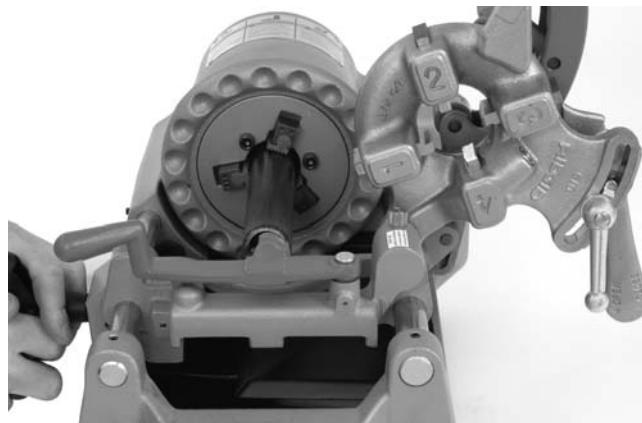
**Figure 12 – Reaming Pipe with No. 334 Reamer**
