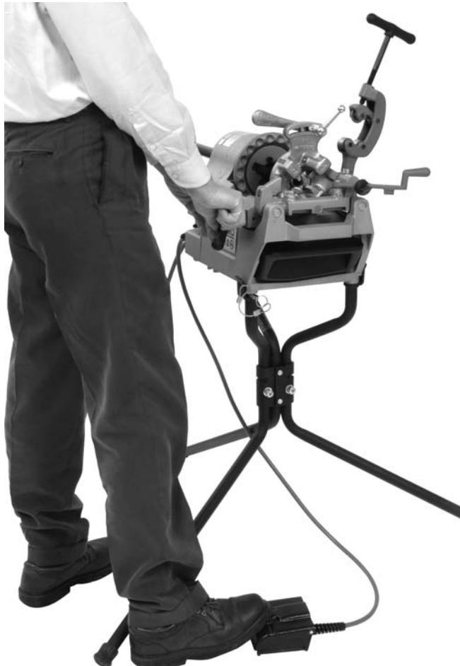
**Figure 10 – Operator in a proper operating position**
