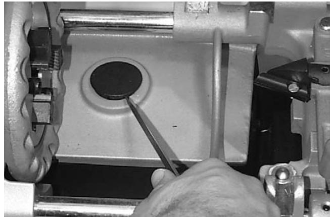
Figure 18 – Removing Brush Cap Plug
