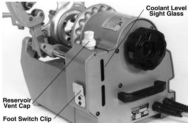
**Figure 1B – 1210 Threading Machine**
