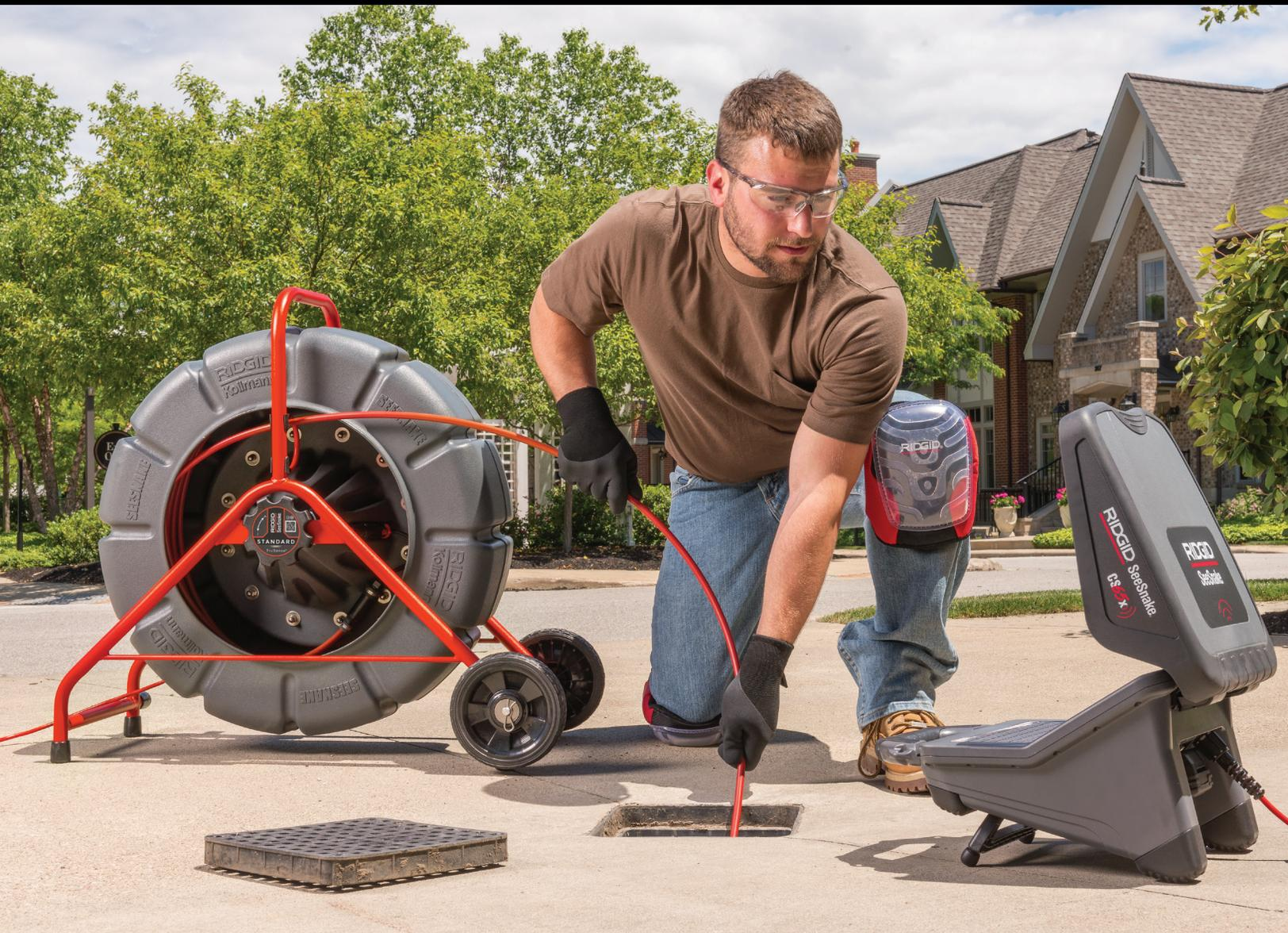
Equipped with the largest diameter SeeSnake® camera head, the Standard is your go-to machine for inspecting long runs in main sewer laterals. Everything about the Standard suggests durability, from the all-metal frame and hardened stainless steel camera head to the stiff cable. Newly available TruSense technology provides a high dynamic range (HDR) image sensor and a TiltSense™ inclinometer for SeeSnake CSx series Wi-Fi enabled monitors.
