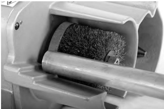
Figure 12 – Deburring O.D. Of Tube
