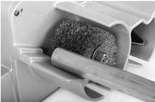
Figure 11 – Cleaning Tube O.D.
