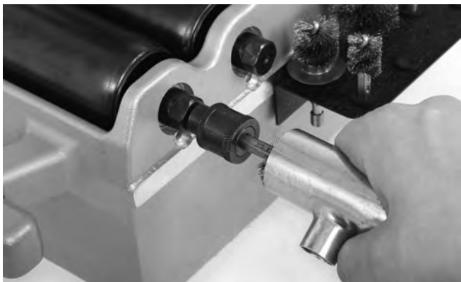
Figure 14 – Cleaning Inside of Fittings
