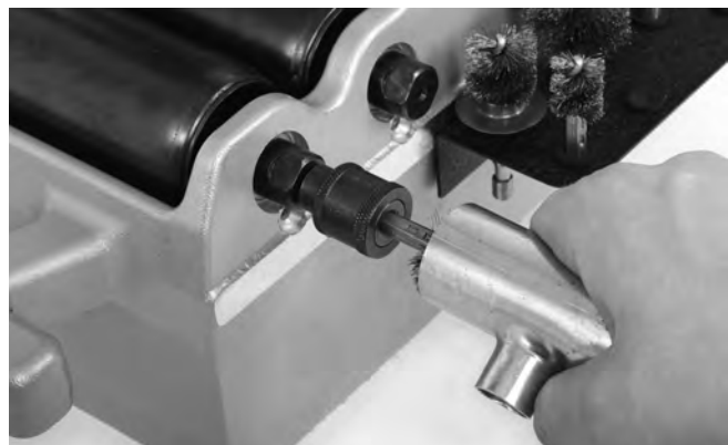
Figure 14 – Nettoyage interne des raccords
