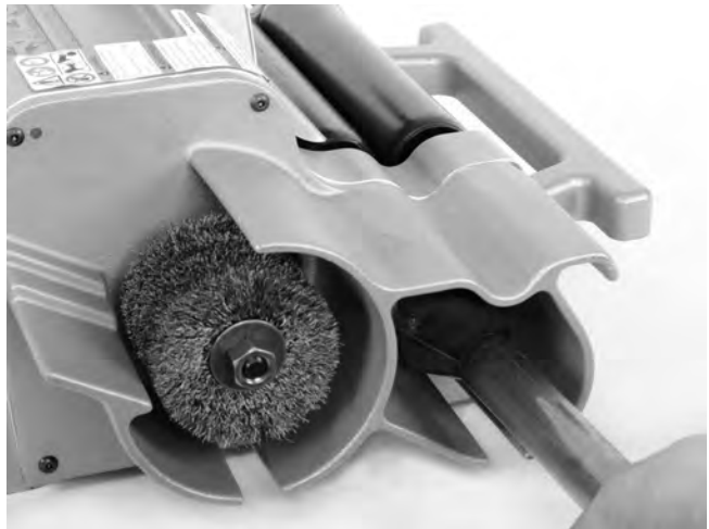
Figure 13 – Reaming I.D. of Tube
