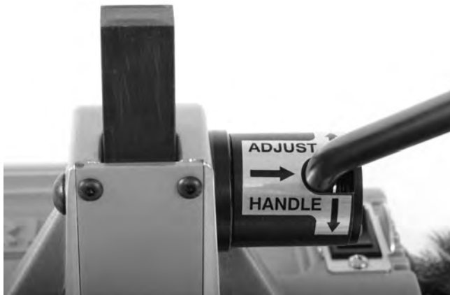
Figure 8 – Adjusting Handle Position
