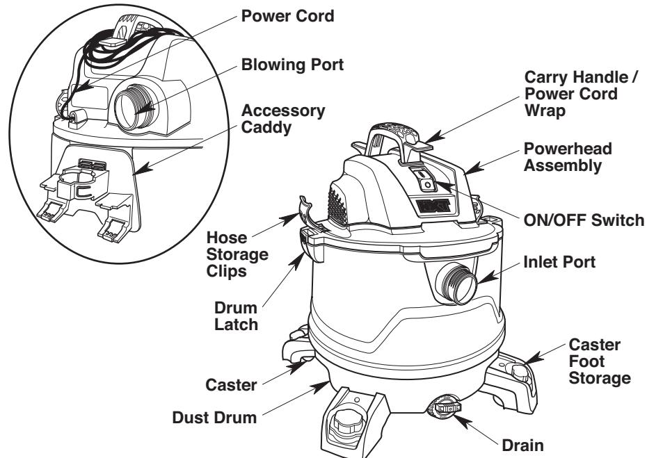
Familiarize yourself with the accessories included with the Vac. Each accessory may be used in various ways for vacuuming and blowing debris. Here is a list of the accessories and their uses.
