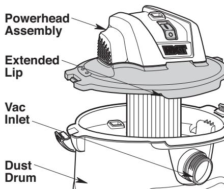
2. Press in on the two Latches located on either side of the Dust Drum until they snap into place, securing the Powerhead Assembly to the Dust Drum.
