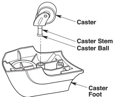
4. Place Caster Foot with Caster over post on bottom of Dust Drum and press firmly in place, as shown.
