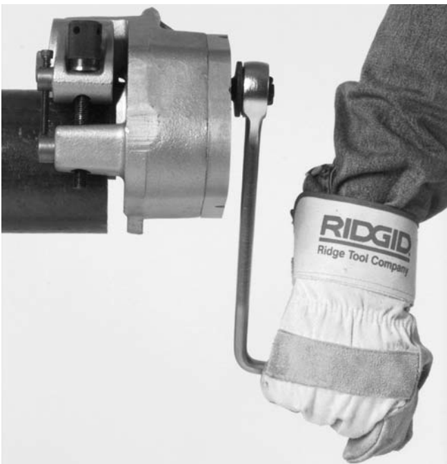
Figure 6 – Rainurage du tuyau
