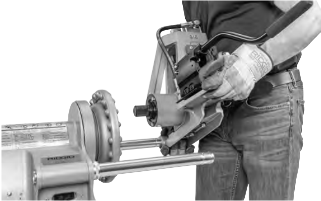
Figure 7A – Installing 918 on 300 Power Drive
