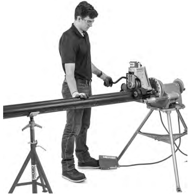
Figure 20 – Applying Pressure on Pipe with Power Drive in FOR direction
