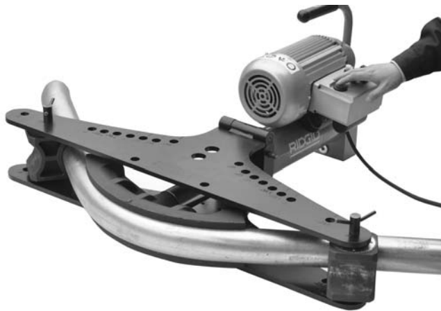
Figure 14 – Operating the Electric Bender
