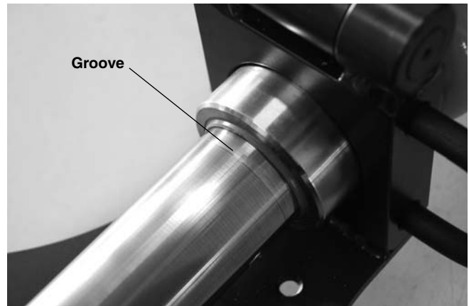
Figure 16 – Groove in Ram
