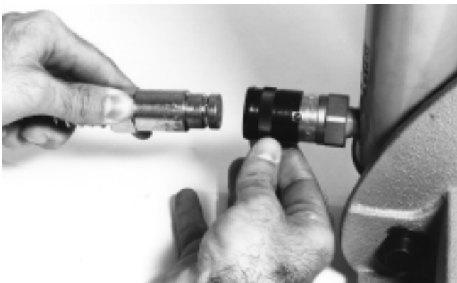
Figure 3 – Connecting Hydraulic Foot Pump to Cutter
