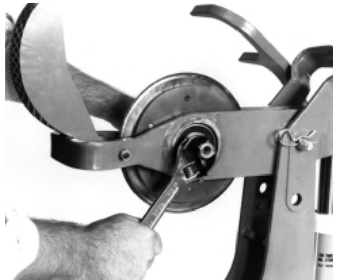
Figure 11 – Remove Locking Nut
