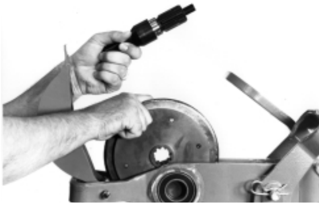
Figure 12 – Remove Cutter Wheel Assembly
