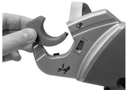
Figure 7 – Installing Multi-Layer Pipe Support Adapter
