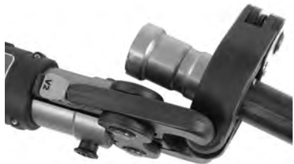
Figure 12B – Placing Actuator Into MegaPress Ring Pockets At An Angle For Additional Clearance
